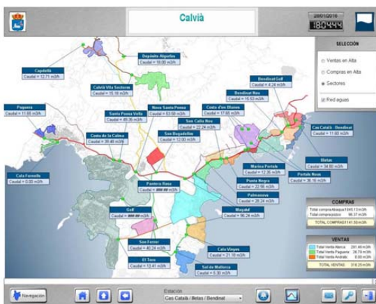
Pantalla general TELECONTROL
